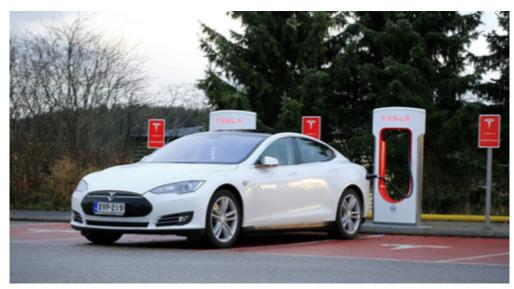
Fast recharging is just one additional plus with Lithium Ion cells. Tesla's SuperCharger system, shown here, can provide 100 miles of range on 30 minutes of charging. Image credit: Taina Sohlman/shutterstock.com
